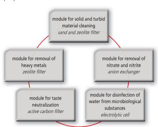
The Disinfection of water from microbiological substances is performed by a specially-developed electrolytic cell with diamond electrodes. Different versions allow the use in the industrial and private sector.
